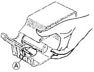
1. Open the right cover. Then push the head-up lever in the direction indicated by the arrow.
